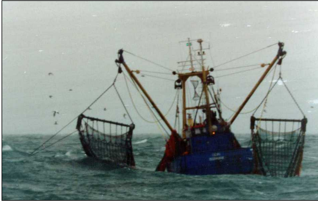
Figure 29. Beam trawler snagged on out-of-use cable.
