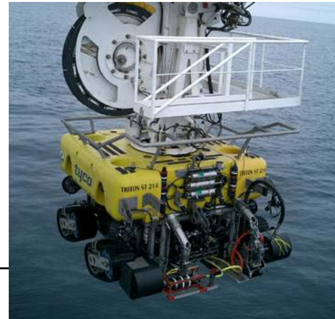
ROV with Jetting
