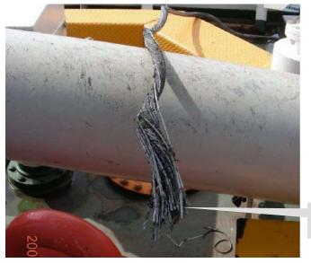
Using ROV the cable was found to be pulled north of it's original as-laid position. Severe serving damage was found as the ROV approached the break. There were large quantities of debris nearby and over the cable including an anchor.
