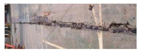
Cable was out of position by approximately 400 meter to the North of the as-laid route. The cable showed signs of external aggression and appeared that the armor wire was embedded into the polyethylene jacket causing the shunt fault.
