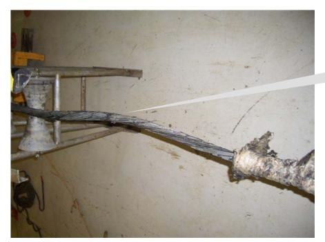
Exposed armor wire and stress, possible fault location
