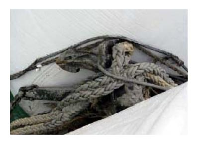
Large Anchor (1.6 Tons) hooked the cable and dragged cable until mooring line of anchor parted or was cut. The Anchor and cable came up to the Aft Deck of the repair ship with submarine cable entangled.
