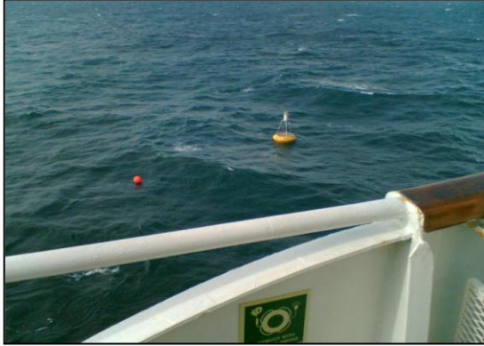
Figure 6: "Cable repair buoy placed by cable ship." Courtesy BT
