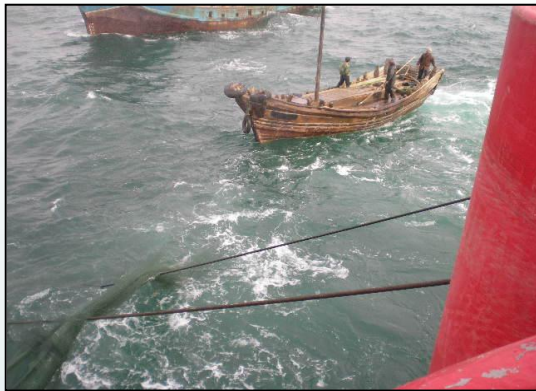
Figure 4: "Fishing vessel, ignoring 1 nautical mile safety margin, with nets entangled on cable, interrupting cable repair." Courtesy SBSS
