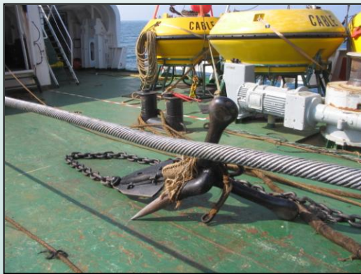
Figure 5: Cable repair buoys on cable ship deck." Courtesy BT
