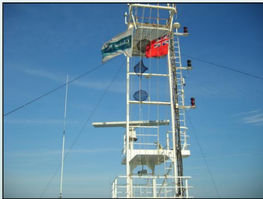
Figure 3: "Cable ship exhibiting COLREG day shapes for vessel with restricted maneuverability." Courtesy GMSL
