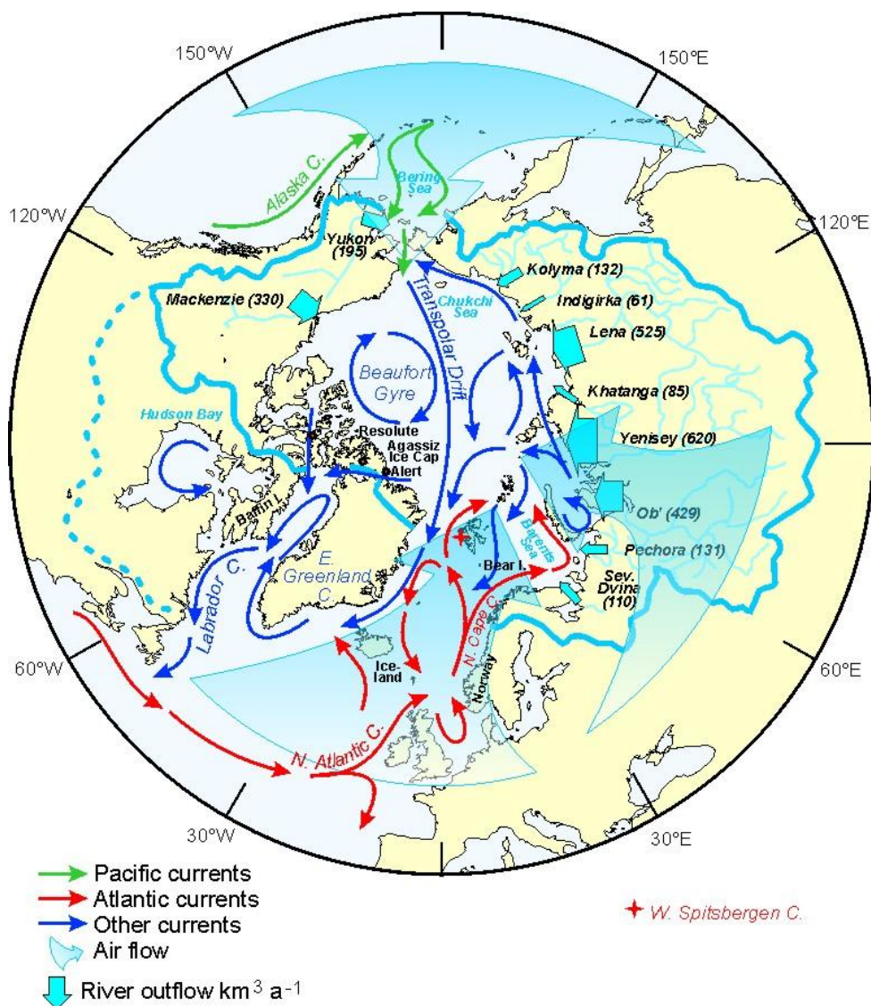
Figure 6.1. Long-range Transport Mechanisms of Pollutants to the Arctic
