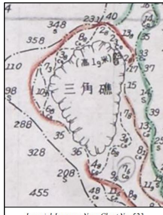
Imperial Japanese Navy Chart No. 523 (depicting sand cay with height of 1.9 metres above Mean Sea Level)
