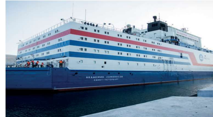
Floating NPP, Russia 2x35 MWe PWR In Operation
