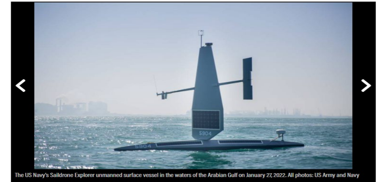
The US Navy's Saildrone Explorer unmanned surface vessel in the waters of the Arabian Gulf on January 27, 2022. All photos: US Army and Navy
