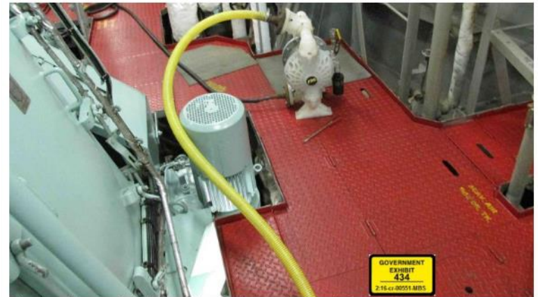
The alleged “magic pipe” discharge line found aboard the chemical tanker Green Sky (file image courtesy USCG)
