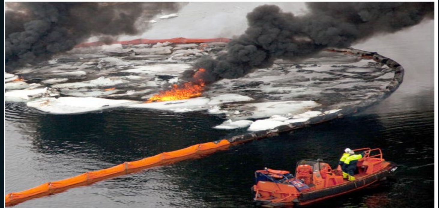
Responding to oil spills in the ice-covered Arctic Ocean would pose unique challenges. For example, floating booms often used to concentrate oil for burning—as in this field experiment in the Barents Sea—must be strong enough to handle increased drag from ice floes. Photo courtesy SINTEF .
